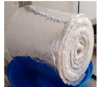
Photo of Aerogel Flexible Sheet Roll
